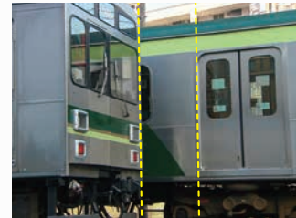
No Rolling Shutter Artifacts with Global Shutter
